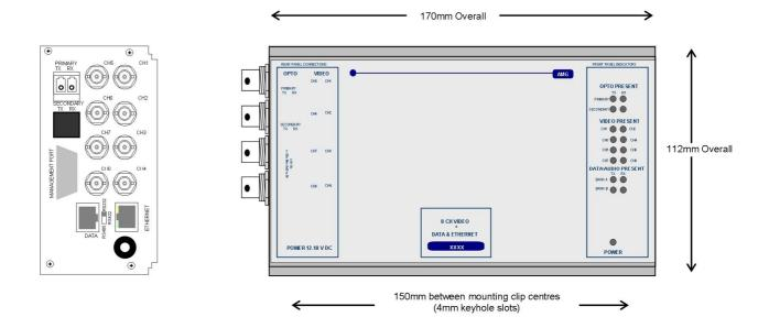
The **AMG4683E-SF** is a standalone eight channel video transmit unit designed to transmit 8 video signals and transmit and receive 1 data signal plus full duplex 100BaseT Ethernet connectivity over one Multimode fibre.
